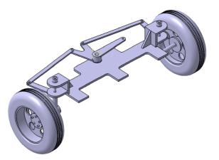
Figure 5: CAD representation for a 3D rear steering linkage mechanism.
